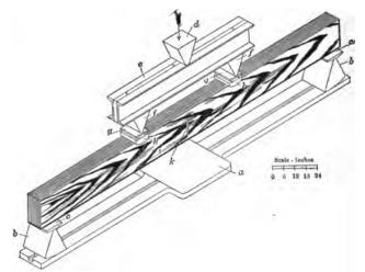
Fig. 3.—Bending test,  $8^{\prime\prime}\,\times\,16^{\prime\prime}\,\times\,16^{\prime}$  bridge stringer.
